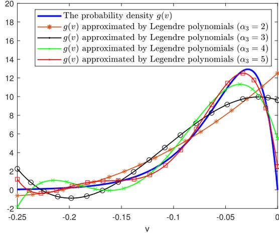
Fig. 4.  $g(v)$  and  $\hat{g}(v)$  with  $\alpha_3 = 2, \dots, 5$ .
