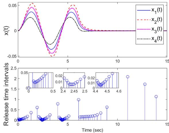
Fig. 3. State responses  $x(t)$  and release instants for  $\alpha_1 = \alpha_2 = \alpha_3 = 2$ .
