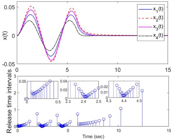
Fig. 2. State responses  $x(t)$  and release instants for  $\alpha_1 = \alpha_2 = \alpha_3 = 1$ .
